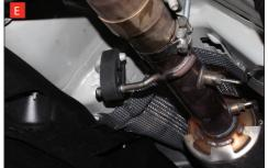
Before removing the original system disconnect the exhaust valve.
